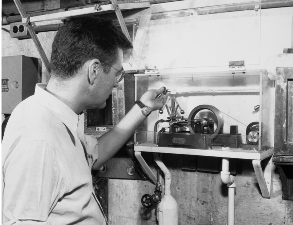
Logan Emlet with toy steam engine which using steam produced by the Graphite Reactor turned a generator to produce the world's first electricity from a nuclear reactor
