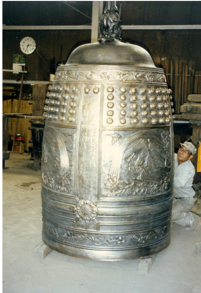
Finished bell fresh out of the casting mold with finishing touches being applied
